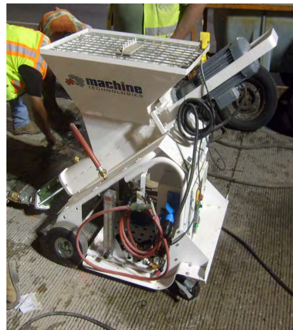
Volumetric Mixer Pump (continuous mixing and pumping)
