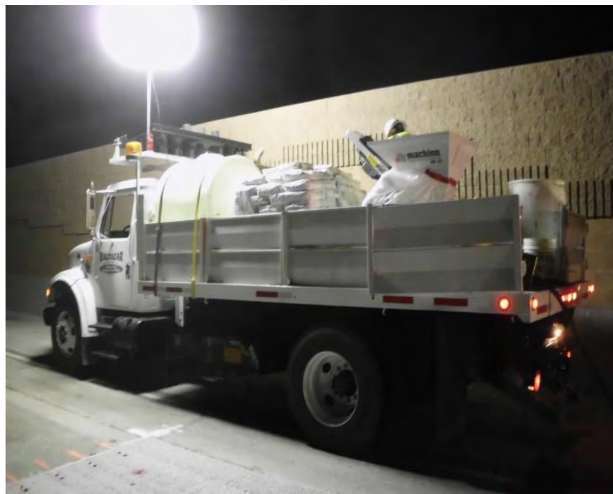
Truck-Mounted Grout System
